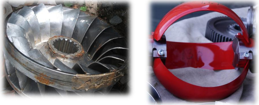
Figure 1 - Comparison of the design of the radial-axial (left) and orthogonal (right) turbine
